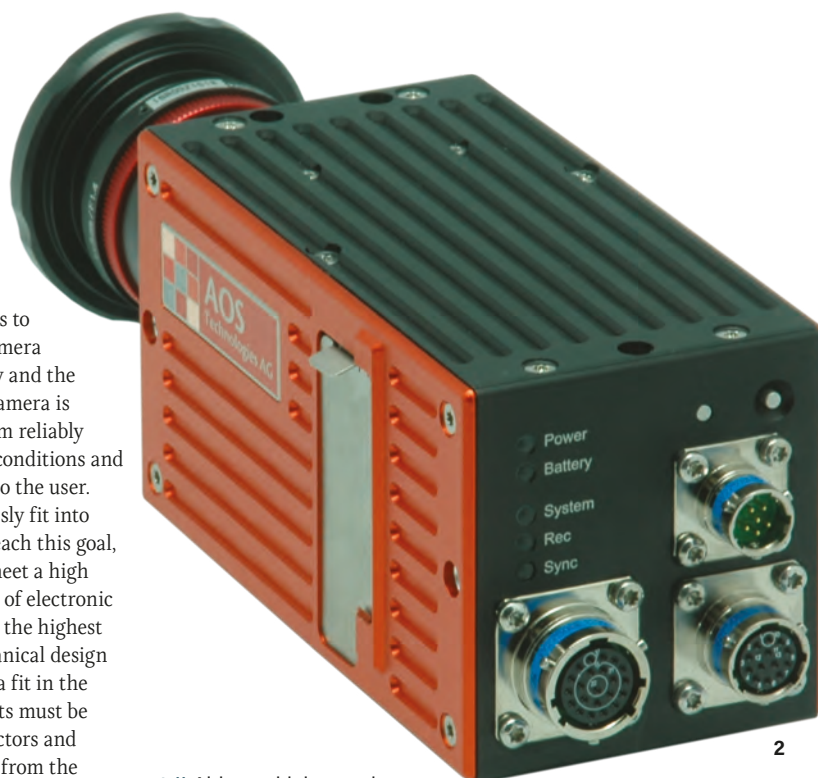
1 // Airborne high-speed camera with recessed lens mount and CFast memory card slot
