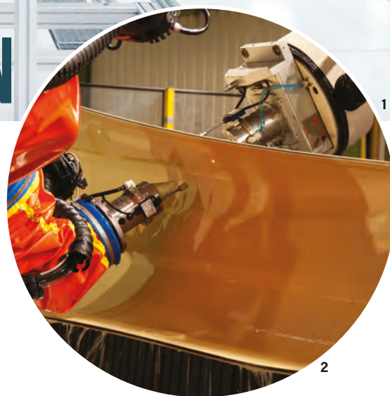
1 // A Tecnatom robotic system inspects a part from Corse Composites
