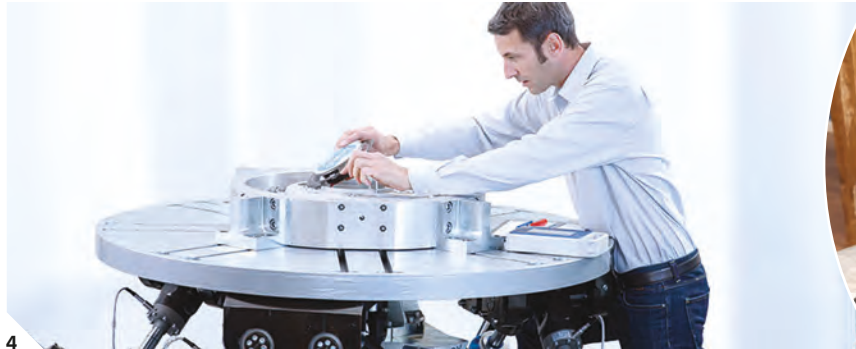
4 // Automatic calibration on hydraulic hexapod at Kistler
