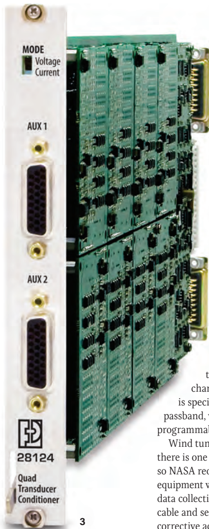
3 // A Precision Filters 28124 Signal Conditioning system card
