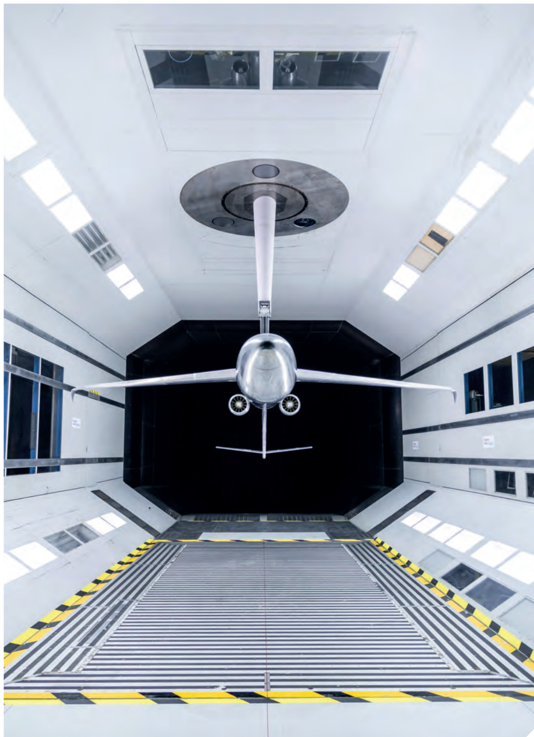
4 // Green Regional Aircraft model equipped with turbofan engines developed and manufactured by the ESICAPIA consortium
