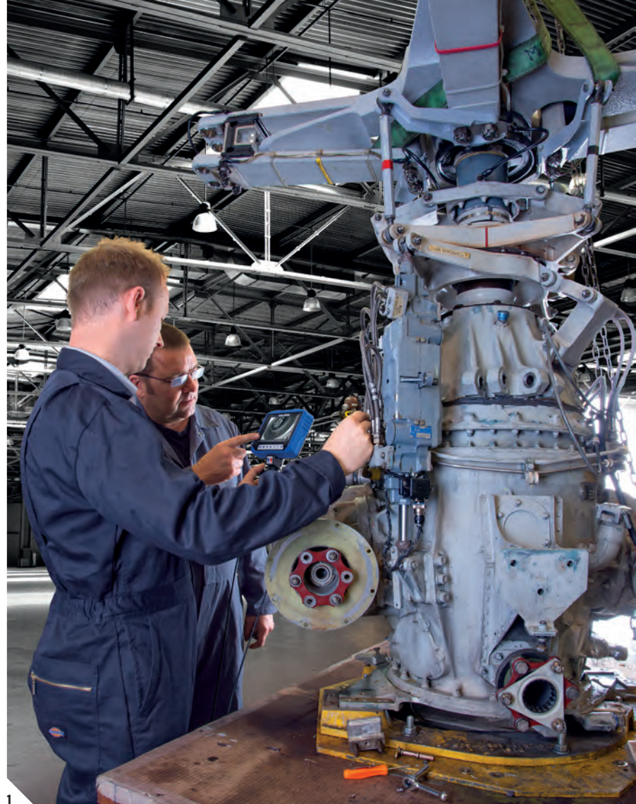
1 // Remote visual inspection of a helicopter gearbox using the portable MoVeo videoscope from Karl Storz
