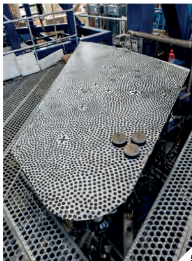
5 // Upper surface digital image correlation paint scheme for strain comparison with strain gauges and fiber-optic strain sensor
