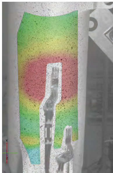
FAR LEFT: Aramis delivers measuring data for part geometries as well as three-dimensional displacements and provides information about the behavior of the components under load
