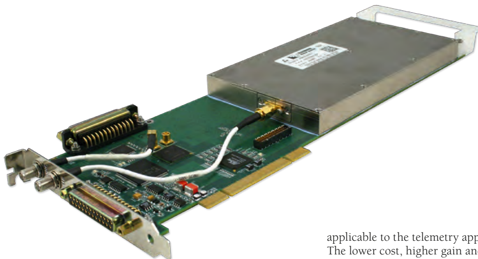
ABOVE: The RMDS-500S-8 C-band PCI receiver
