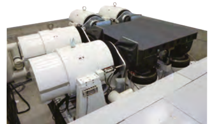
6 degree of freedom vibration test system
