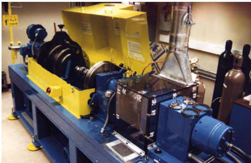
ABOVE: Sub-scale aircraft brake dynamometer (model 2076 by Link Engineering), 7,000rpm capacity, adjustable inertia (0.27 and 6.37 kg•m 2 ), maximum normal force of 13.3kN, and maximum torque of 34.6 kg•m
