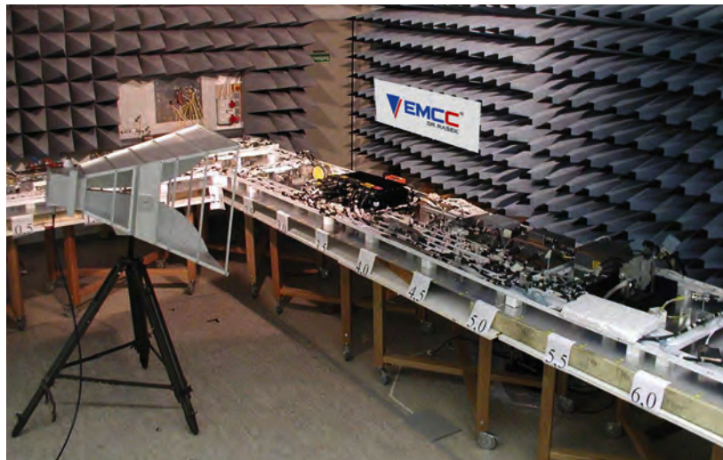
ABOVE: A test bench for testing electromagnetic compatibility
