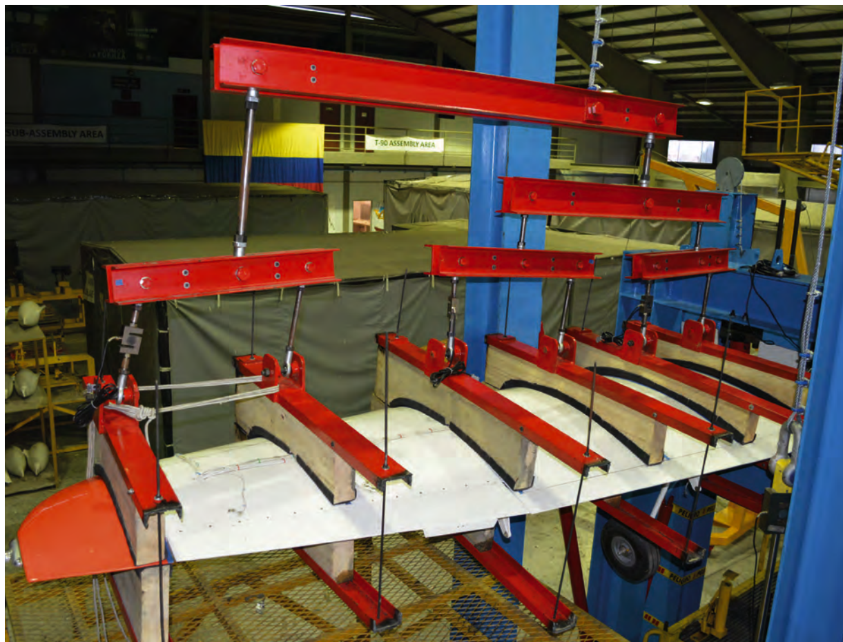
LEFT: The wing plane of the Calima T-90 exceeded the ultimate load for more than three seconds and showed to be very safe for the critical flight conditions, reaching 6.3g at a very critical load condition
