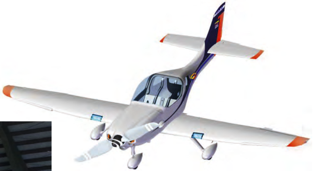
ABOVE: More than 90% of the Calima T-90's structure is constructed in carbon and glass fiber-reinforced polymer
