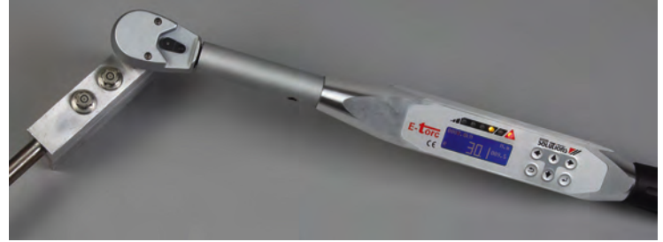
ABOVE: Wrench displaying load, torque and angle on the handle
