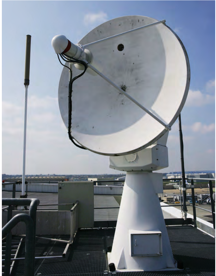
ABOVE: Airbus uses a C-band telemetry system for the transmission of test data
