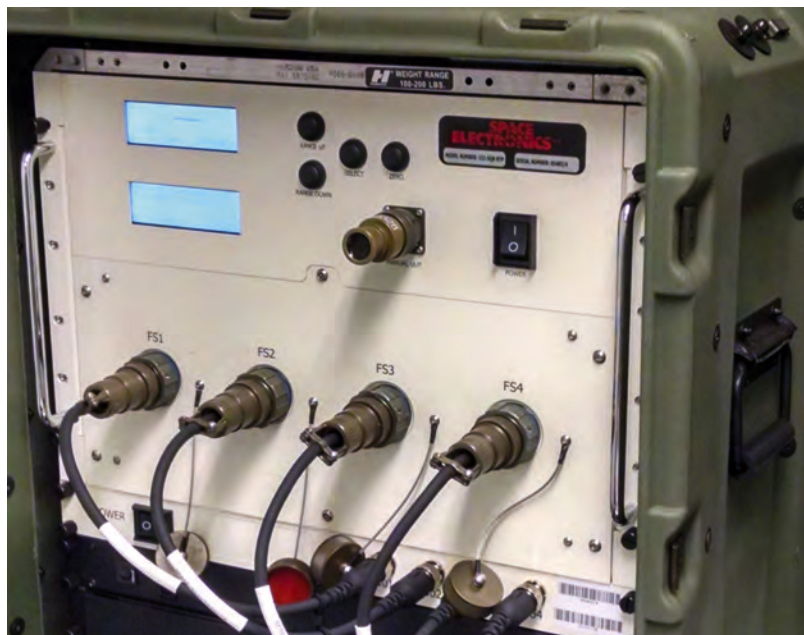
ABOVE: Model 132-SQB-BTP 32 test point circuit tester
