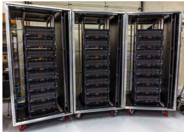
FIGURE 5: 768-channel system front-end units
