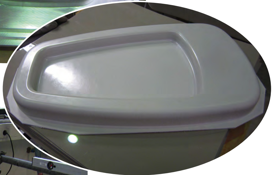
BELOW: Upper panel made from the tooling, shown before trimming
