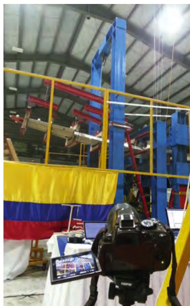
RIGHT: The wing plane of the Calima T-90 was subjected to a first stage equivalent to 4.05g, while the operation of the control surfaces were tested
