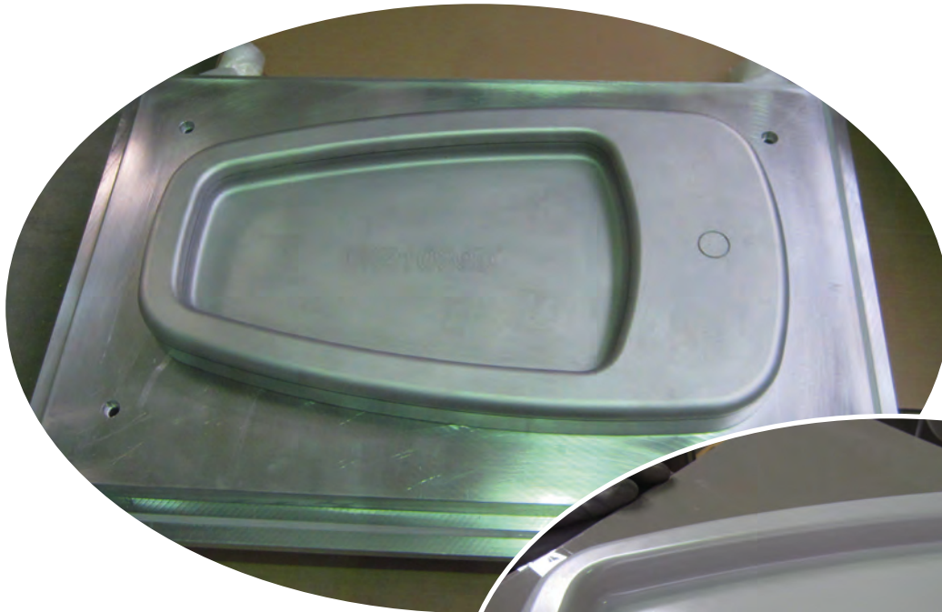
LEFT: Tooling for molding the upper panel of the unit
