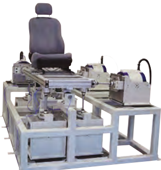
6 degree of freedom vibration test system
