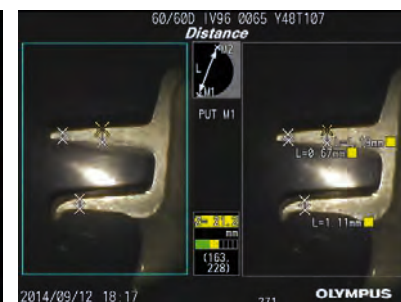
ABOVE: (L) Standard videoscope – red areas cannot be measured. (R) IPLEX NX with super wide field 3D stereo measurement
