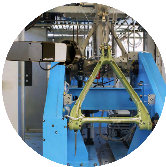
ABOVE: The new landing gear – placed within an individually designed test rig at Liebherr-Aerospace's testing facility in Lindenberg
