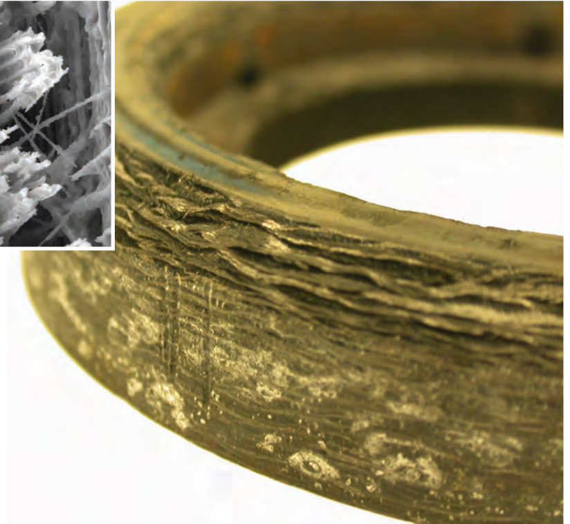
RIGHT: A macro image of 2D carbon-carbon material after being exposed to salt water during simulation testing using normal landing energy
