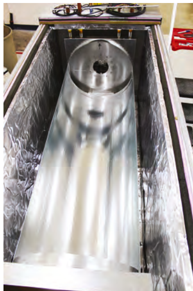
ABOVE: Custom horizontal thermal-cycling chamber (24in diameter by 72in long; 120°C to -235°C at 15°C/minute)
