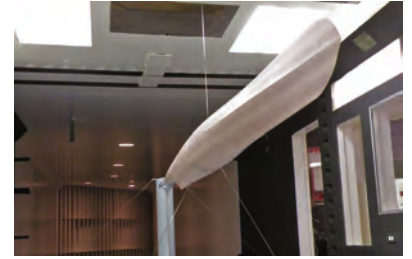
ABOVE: A special mounting system to minimize interference of the support system on the skin friction drag of a trimaran
