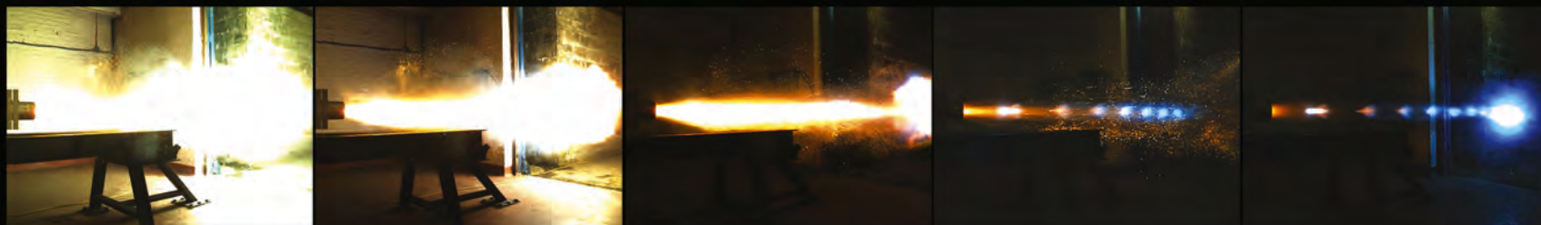
Shock diamond formation in the rocket plume - courtesy of The Falcon Project Ltd.
