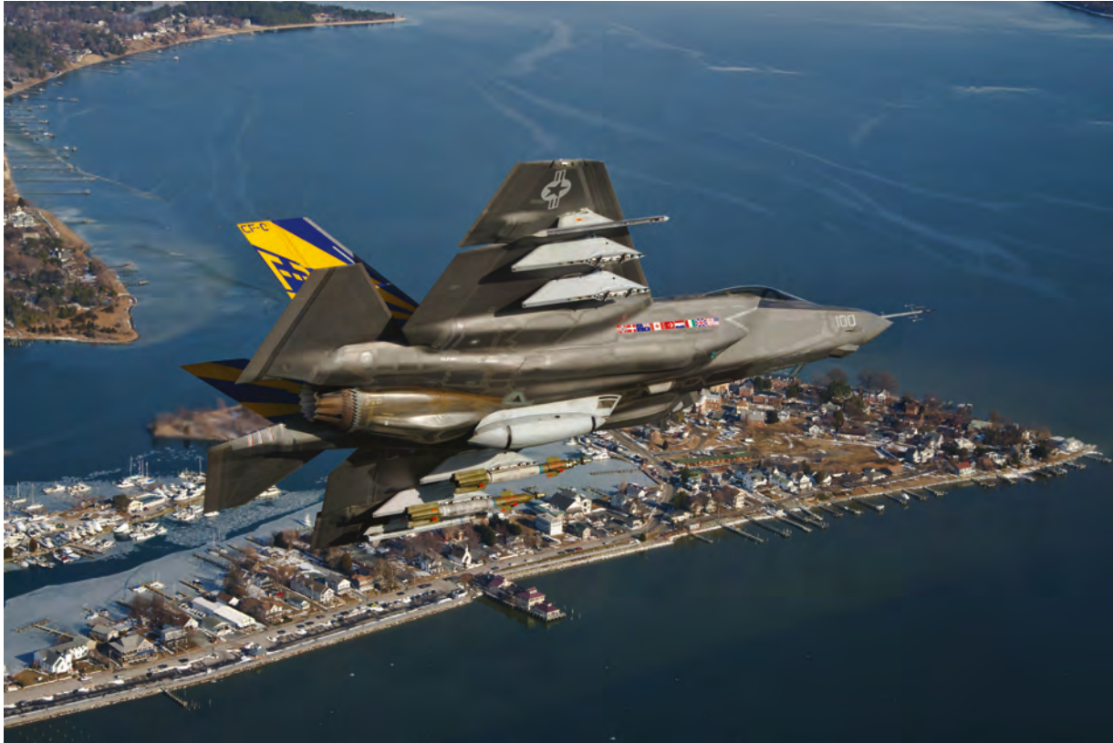
LEFT: During flight 336 of aircraft CF-01 on February 25, 2015, Major John Dirk conducts an F-35C Lightning II asymmetric external stores flying qualities test above NAS Patuxent River
