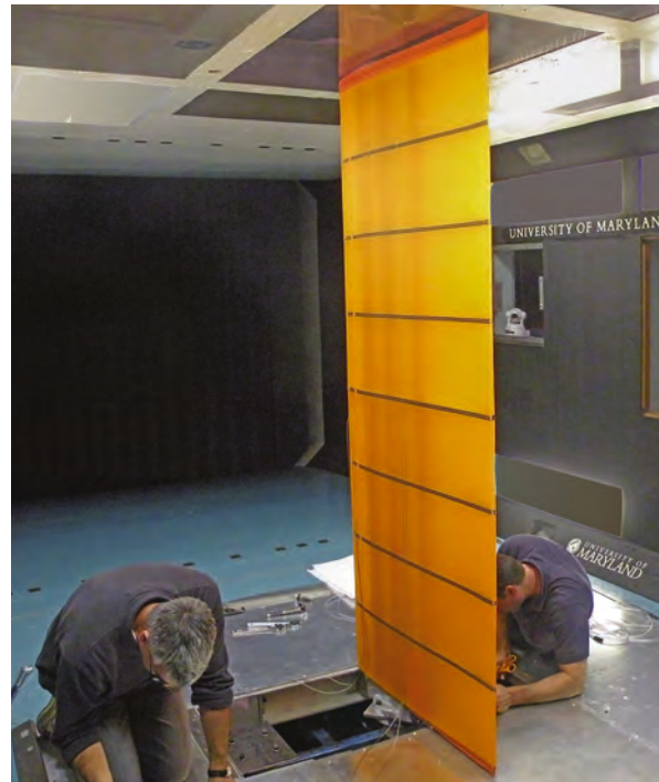
ABOVE: A special mounting system to minimize interference of the support system on the skin friction drag of a trimaran
