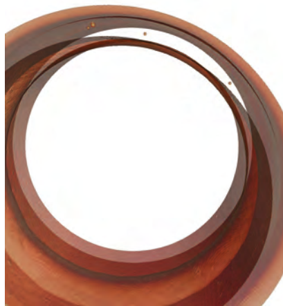
ABOVE: A CT reconstruction of this welded area reveals distinct gas holes, and can accurately locate and measure each indication for disposition
