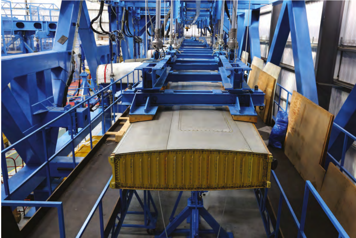
LEFT: The actuators in the wing fatigue test rig apply load to the test specimen along with an airbag loading system
