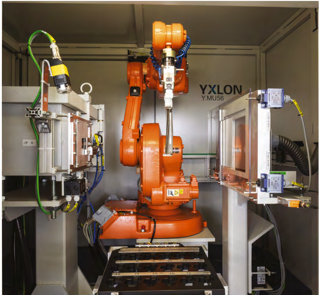
ABOVE: The robot manipulates the turbine blades to the different inspection positions between the x-ray tube and detector
