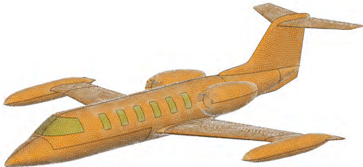
FIGURE 7: The mesh used for the HIRF simulations has 84,579 triangles
