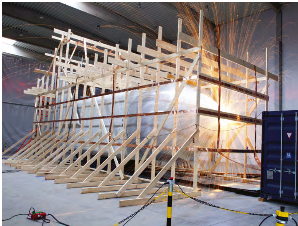
ABOVE: Full-scale test on a nacelle and hub system where the drivetrain is rotating with nominal speed during the test
