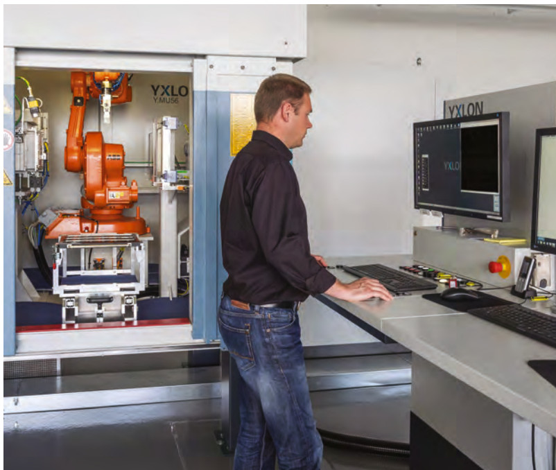
ABOVE: Daniel Genke, an NDT technician at Atlas Air Service, prepares for series inspection of the TiAl turbine blades using the fully automatic Y.MU56 TB x-ray system
