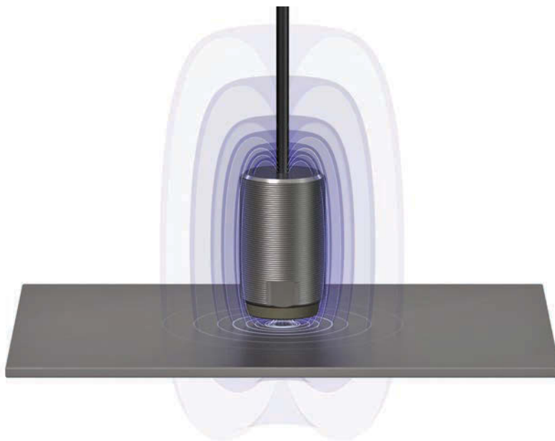
Above: Eddy current measurement principle
