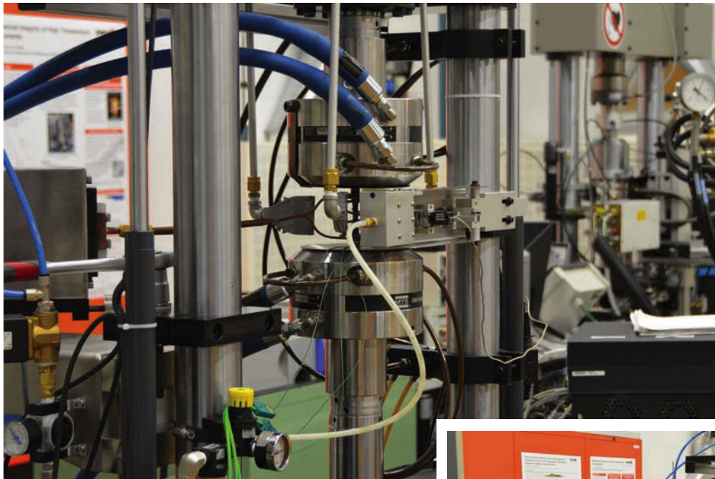
LEFT: Empa's service-cycle component-feature specimen TMF testing methodology requires a test system capable of switching from mechanical strain control to load control within the same cycle, while superimposing high-frequency vibrations
