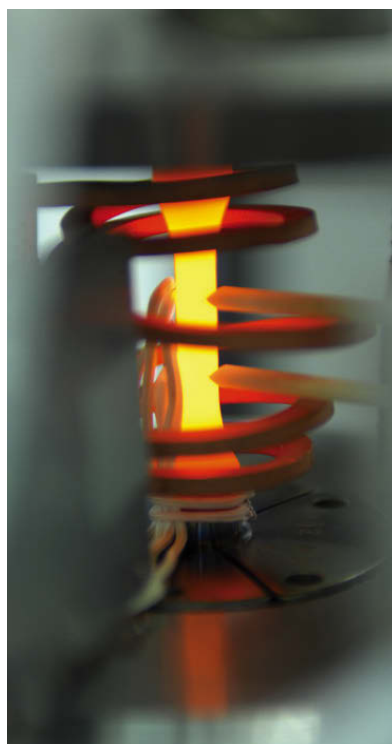
ABOVE & LEFT: Empa's TMF applications require compact, low-mass extensometers capable of running at both high frequencies and high temperatures, and high quality induction coils and enhanced cooling controls to achieve precise temperature control in a consistent, repeatable fashion
