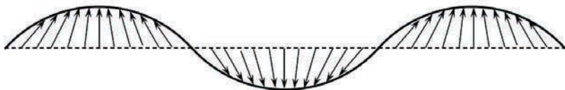
ABOVE: Anti-symmetric mode of Lamb wave (side view of a panel)
