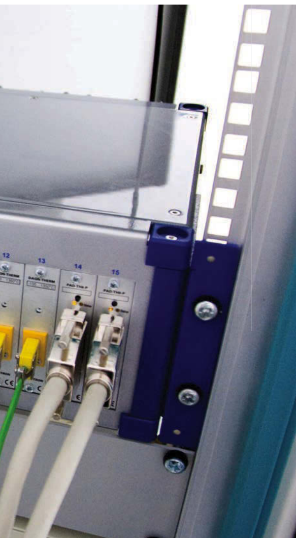
ABOVE: The perfect signal conditioning solution: A DEWE-30-16 with DAQP modules, which have conditioned signal output of either \pm 5V or \pm 10V
