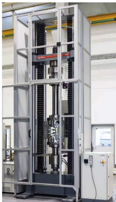
ABOVE: Single column zwicki-Line systems from Zwick deliver accuracy and reliability in uniaxial testing within a space-conserving footprint
