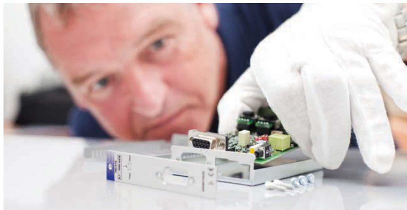
RIGHT: Assembly of a high-speed universal HSI-STG module
