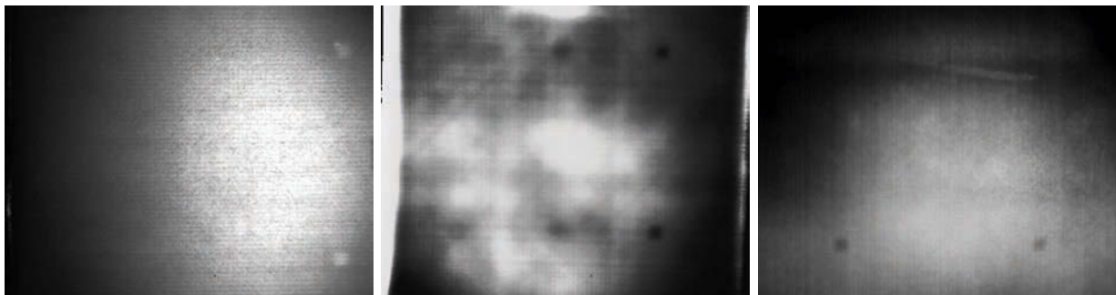
ABOVE: Phase images obtained using a setup of 'error'. From left: Reflection mode (pulse heating: t6); transmission mode (pulse heating: t8); lock-in mode (pulse heating t5, 3 cycles, fadq=20Hz)
