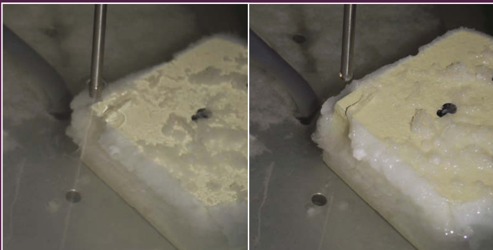
BELOW RIGHT: Fuel has been drained to show the area of erosion
