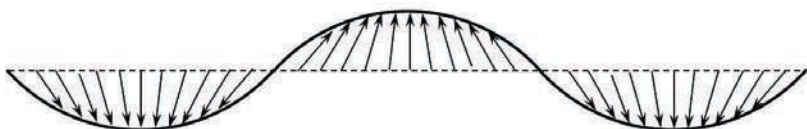
ABOVE: Symmetric mode of Lamb wave (side view of a panel)
