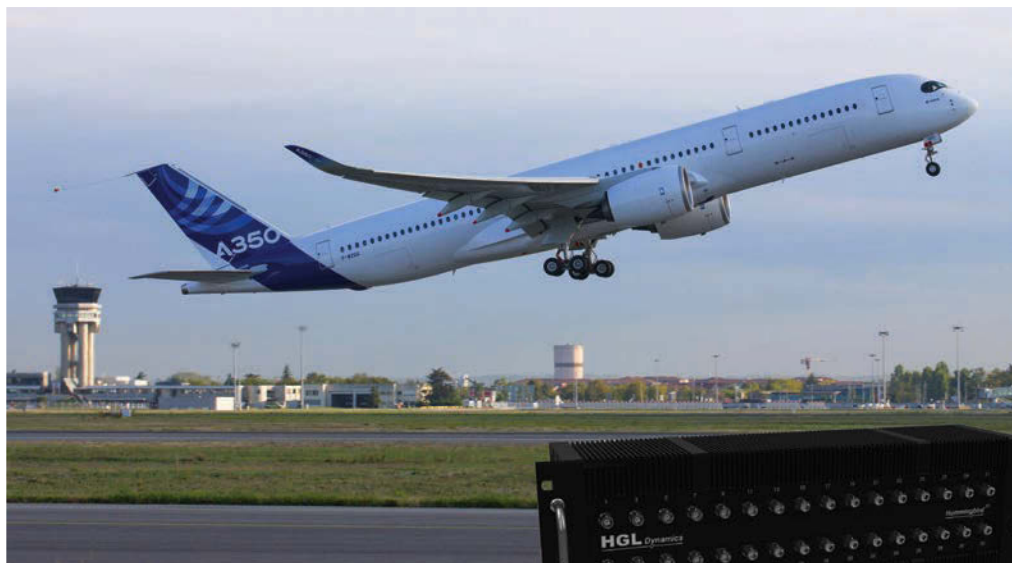
LEFT & INSET: The Hummingbird 32 is currently installed on the A350 flight test aircraft
