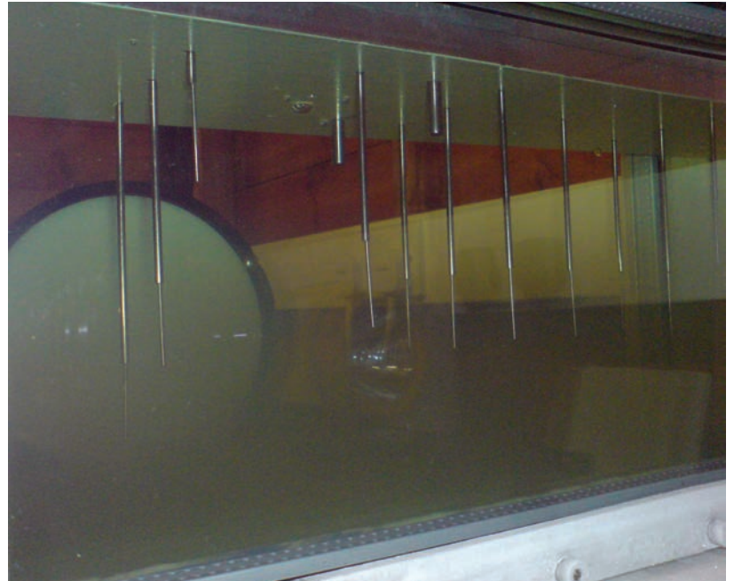
ABOVE: Bottom cooling mode. Cloudiness developed from the bottom of the fuel tank, since heat transfer is dominated by conduction, which leads to a stratified regime
