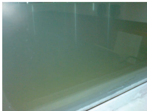
ABOVE: Bottom cooling mode. Cloudiness developed from the bottom of the fuel tank, since heat transfer is dominated by conduction, which leads to a stratified regime
