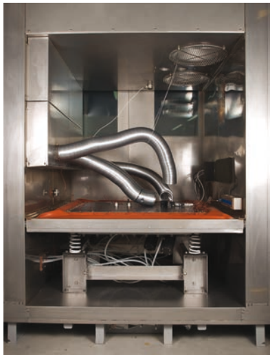
RIGHT: HASS/HALT chamber (Vötsch Model Star Galaxy 36 Premiere)
