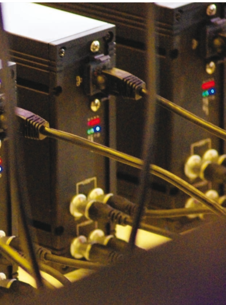
ABOVE: Large, multichannel systems can be assembled from small modules by passing power and synchronisation from one to another
