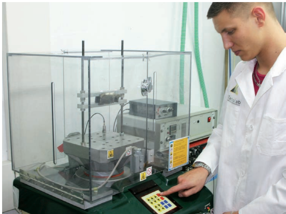
Inputting parameters and factors for shock and vibration tests
