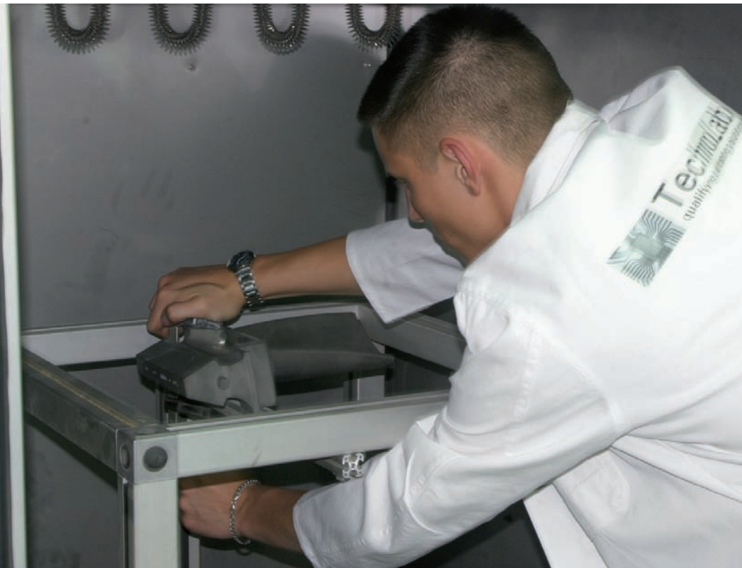
Fastening an object in the chamber for sand and dust testing
