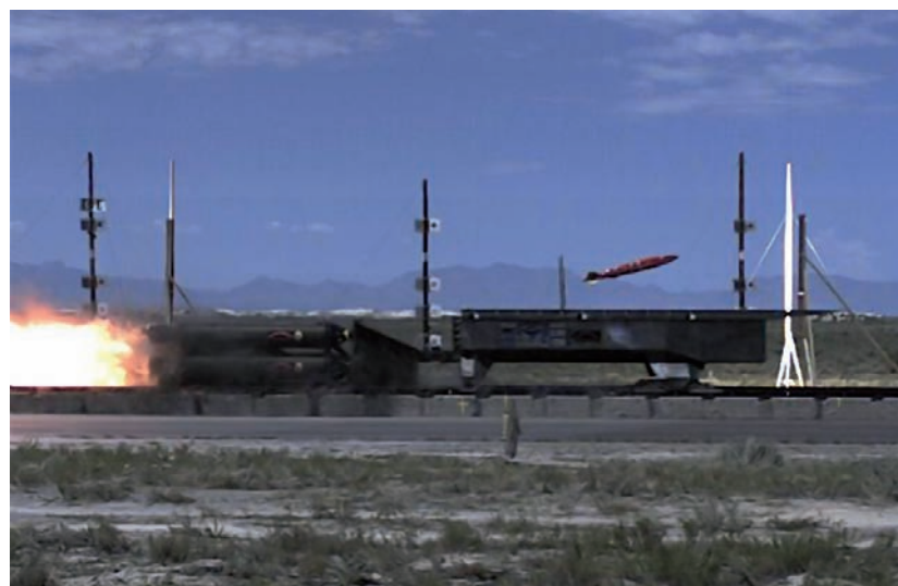
The 10 mile (16km) sled track at Holloman AFB (above). The first-ever test release of an MK-82 Joint Direct Attack Munition on a rocket sled traveling at supersonic speed (right)
