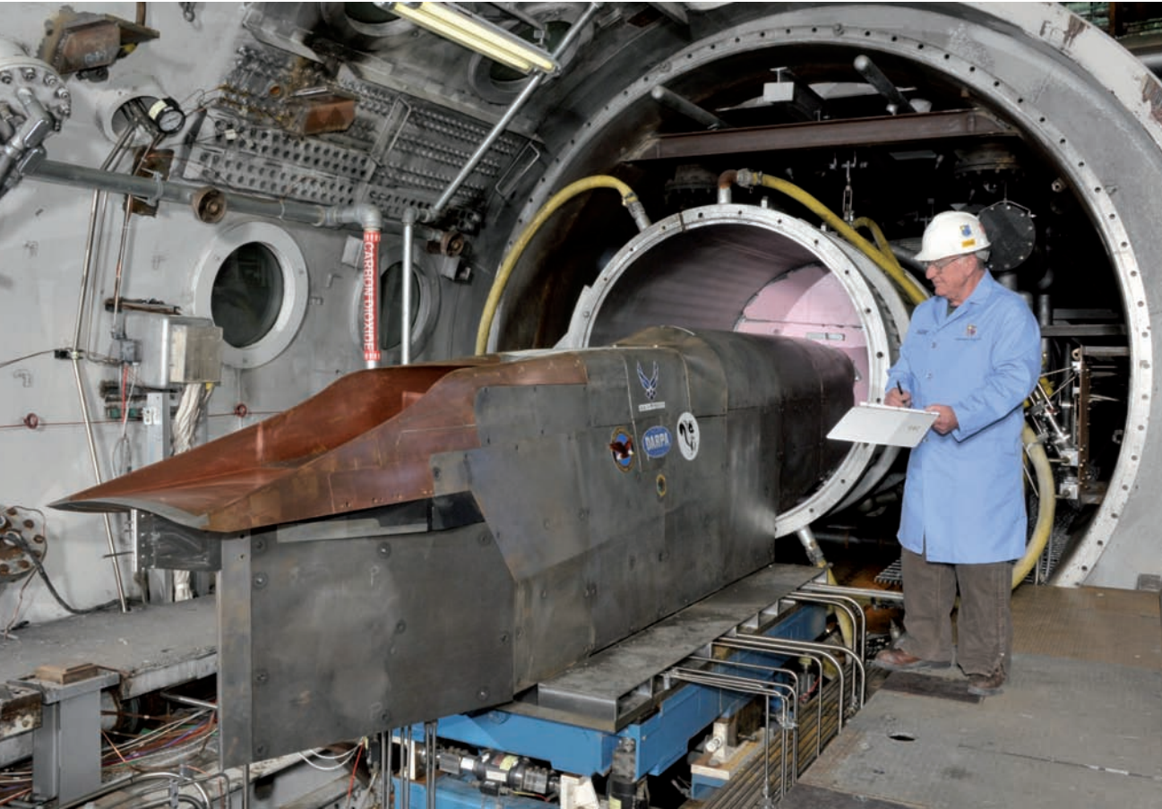
Outside Machinist Everett Fulmer inspects the Defense Advanced Research Projects Agency's Falcon Combined-cycle Engine Technology scramjet test article
