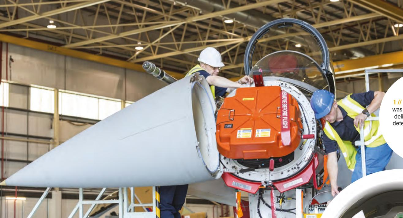
1 // The Typhoon's radar was recently upgraded to deliver a larger array for detection and tracking of threats
