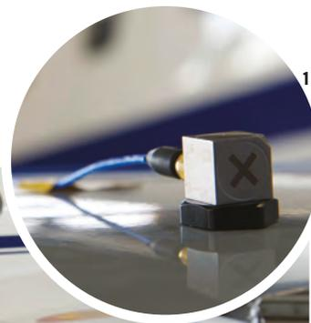
1 // Triaxial ICP modal accelerometer wing mounted with an electrically isolated base
