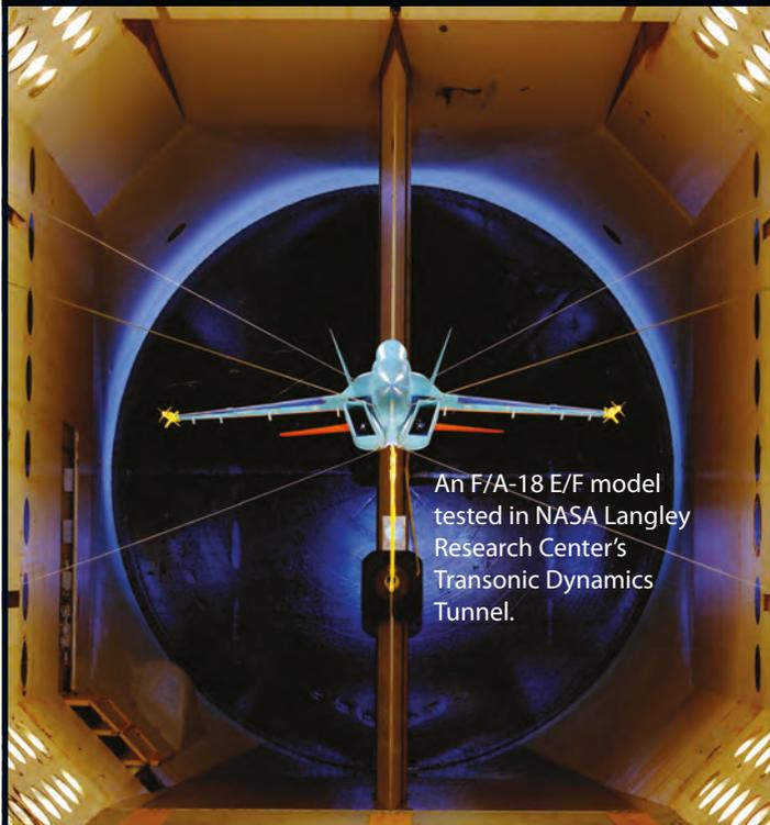
An F/A-18 E/F model tested in NASA Langley Research Center's Transonic Dynamics Tunnel.
