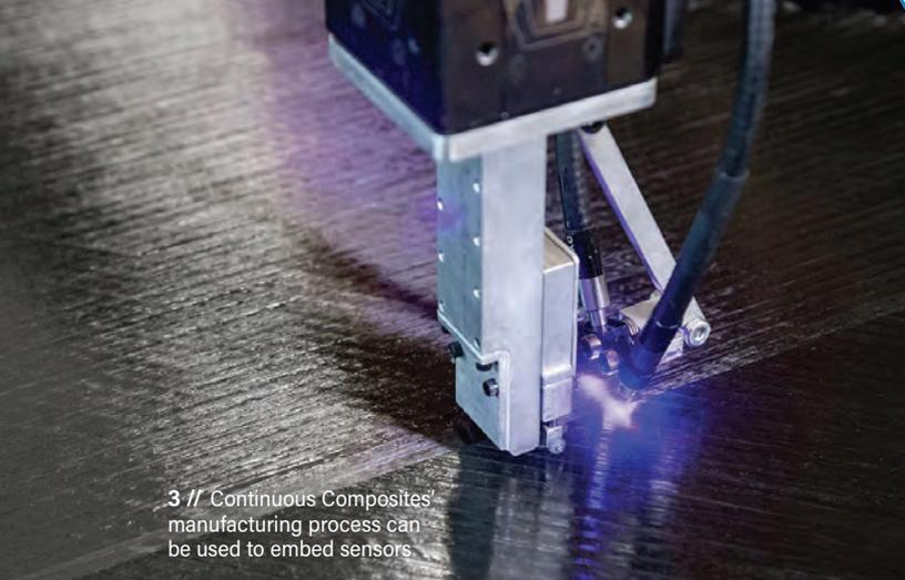
3 // Continuous Composites' manufacturing process can be used to embed sensors
