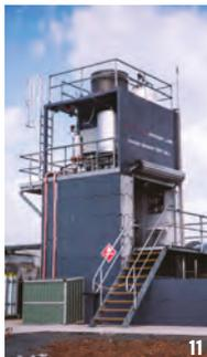
11 // Rocket Lab's rocket engine test cell in New Zealand
