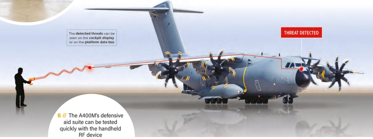
6 // The A400M’s defensive aid suite can be tested quickly with the handheld RF device
