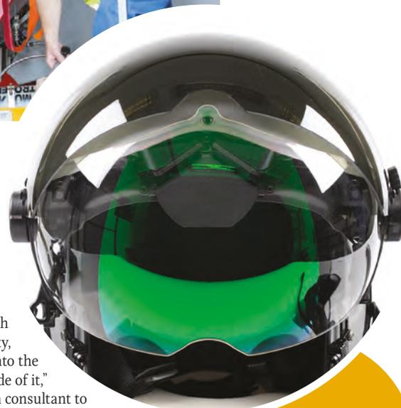
2 // An RAF Typhoon pilot's helmet displays threat information on its visor
