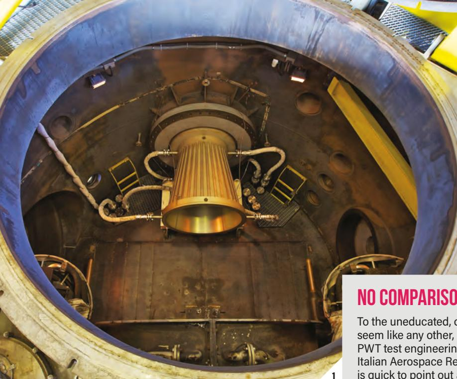
1 // Interior of the Scirocco's test chamber
