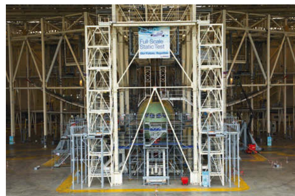
ABOVE: Maximum wing bending test – at ultimate load, the A350 XWB wingtip deflection exceeded 5m
