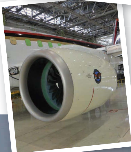
ABOVE: The first PW1200G PurePower geared turbofan engine was delivered to MAC in June 2014 and mounted on the first MRJ90 test aircraft's Spirit AeroSystems engine pylon
