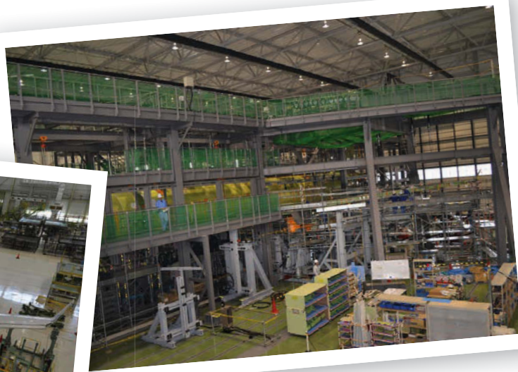
ABOVE: The first MRJ90 airframe installed in the static test rig
