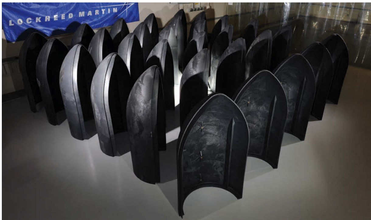
BELOW: Composite rocket nose fairings, made from Lockheed Martin's APEX material
