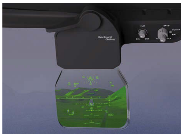
MAIN IMAGE: Rockwell Collins' EVS-3000 offers an uncooled solution that can detect all runway lighting, including new LED systems
