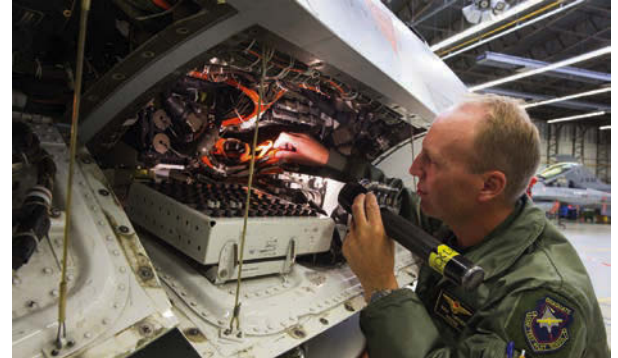
BELOW: 'Lucky' checks out the F-16's orange wiring and new Programmable Master Unit (PMU) in the flight test office hangar
