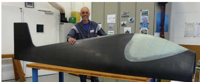
LEFT: The new turtle deck prior to leaving the wind tunnel composite workshop
