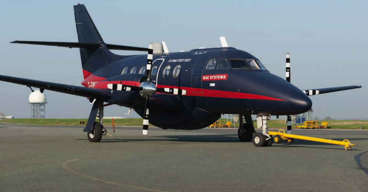
LEFT: BAE Systems' Jetstream aircraft known as 'The Flying Test Bed', which can fly as if it were an Uninhabited Air Vehicle (UAV), has undergone a series of flight trials
