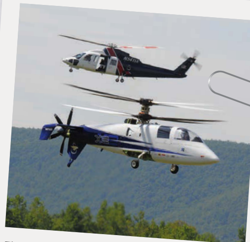
The X2 Technology demonstrator achieved 250kts cruising speed and provided the basis for the S-97 Raider
