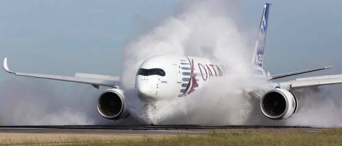
LEFT: MSN004 traveled through troughs containing at least 22mm of water depth, at a variety of speeds, starting at 60kts, and successively increasing to around 140kts, during recent water ingestion testing
