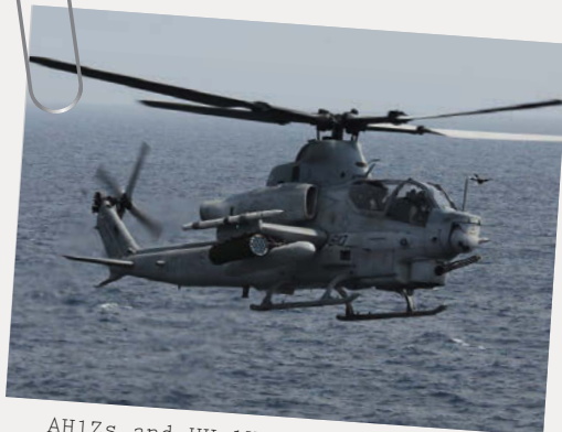
AH1Zs and UH-1Ys underwent software regression and envelope expansion testing in 2010
