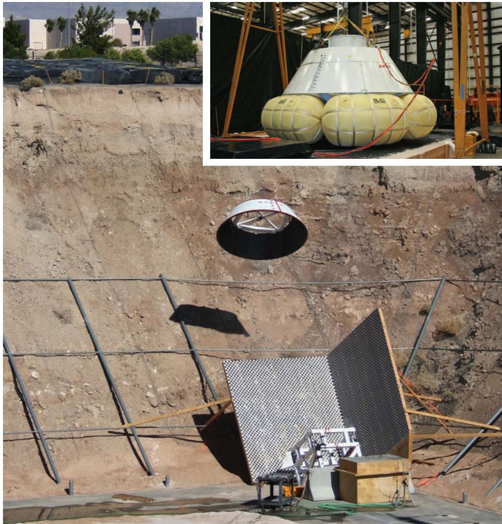
ABOVE: Testing of CST-100 forward heat shield jettison system
