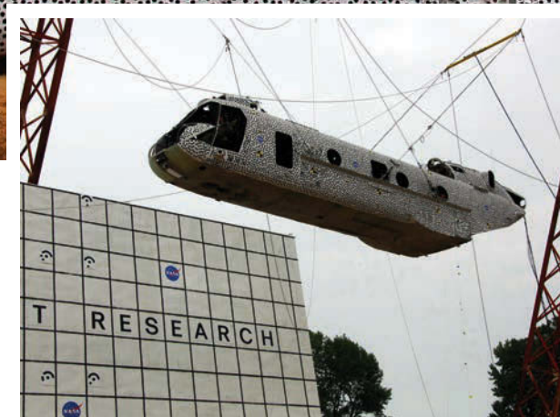
ABOVE: The US Navy CH-46E Sea Knight helicopter fuselage used during the test was painted with over 8,000 dots as part of a high-speed photographic technique
