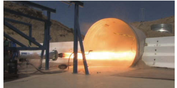
ABOVE: Dream Chaser hybrid rocket motor firing
