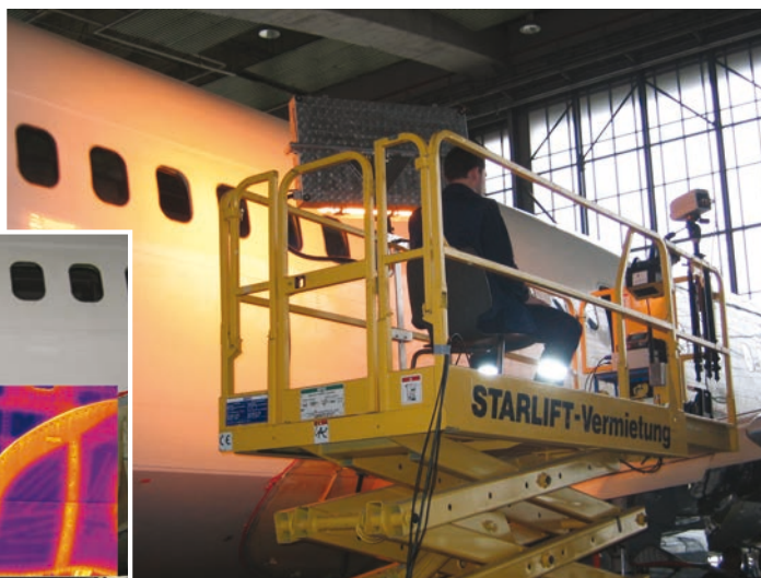
BELOW/RIGHT: Inspection of B737 fuselage. Measurement set-up (right) and fuselage with result images (left)
