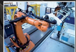
Adaptive Robot Control using Optical CMM or iGPS
