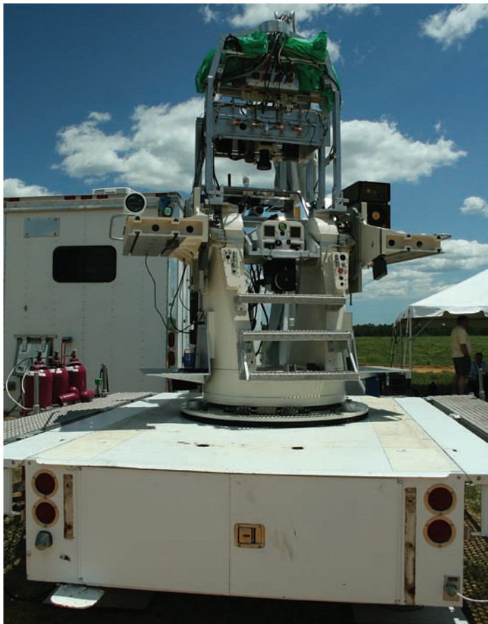
Crane Naval Surface Warfare Center in Indiana built the multi-seeker missile simulator used for CIRCUM live fire test
