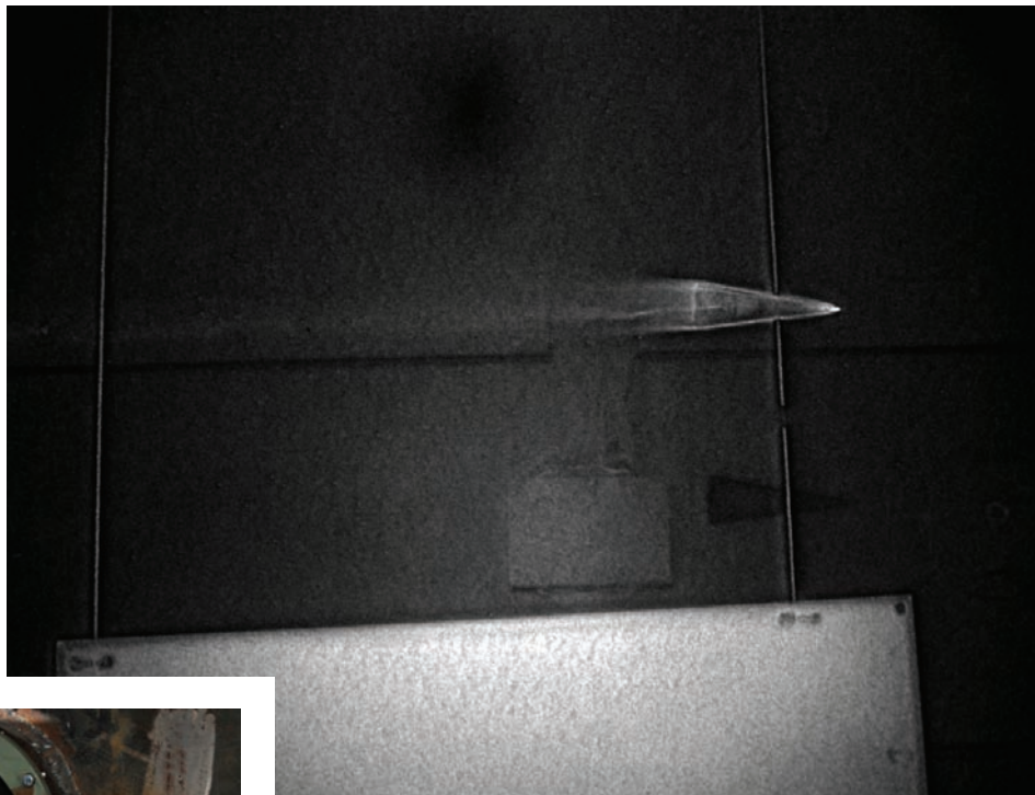
Above: A successful check-out test at AEDC's Hypervelocity Ballistics Range G captured this image of a projectile traveling at 18,000ft a second
