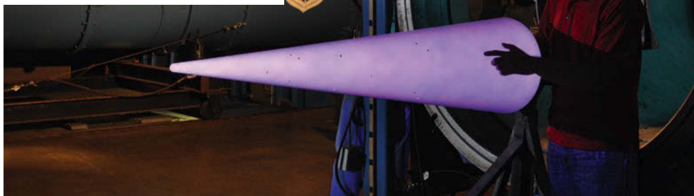
RIGHT: An Air Force project engineer examines the illuminated temperature sensitive paint coating on the large, 7" cone prior to testing (Photo: Mike Smith)
