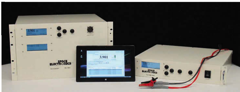
Two automated squib testers: a 16-channel version (left) and a 2-channel version (right)
