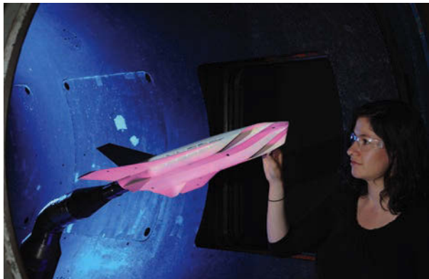
ABOVE: Inna Kurits, AEDC Tunnel 9 test engineer, checks the US Air Force HIFEX vehicle geometry for final readiness before testing in the AEDC Hypervelocity Wind Tunnel 9
