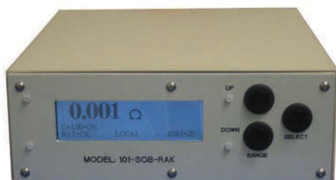
The model 101-SQB-RAK is a single-channel automated squib tester developed for Raytheon and used on the SM3 and ESSM missile programs
