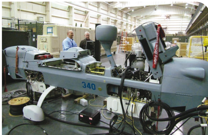
LEFT: An MQ-5 Hunter UAS assembled from the remains of two aircraft that crashed in Afghanistan simulates flight at the UAS Joint Service Integration Lab
