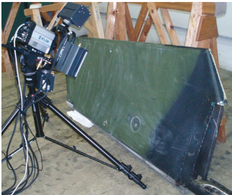
ABOVE AND LEFT: Assessment of a horizontal tail. Left image shows the setup, above shows the image
