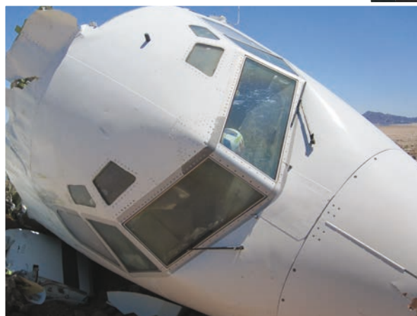
ABOVE: A force of 12g was recorded in the front of the remaining cabin while, further back in the plane, the force dropped to 6g
