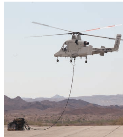
BELOW: At Yuma, the K-MAX moved 33,400 lb over five days, including 3,700 lb in a single mission
