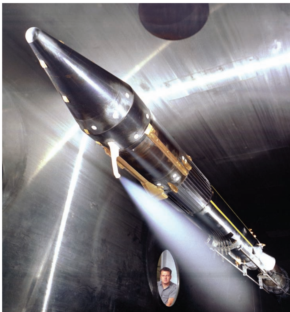
BELOW: Piezoelectric microsensors are small enough to allow multiple installation flush with the surface of the model
