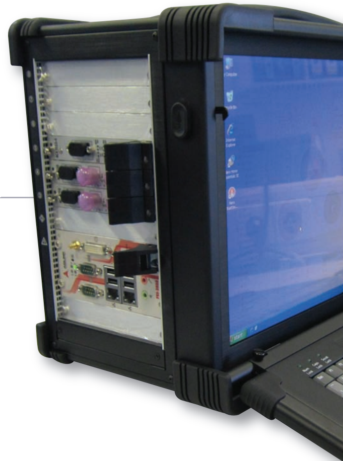
BELOW: Built-in waveform analysis based on a digital scope capable MIL-STD-1553 interface
