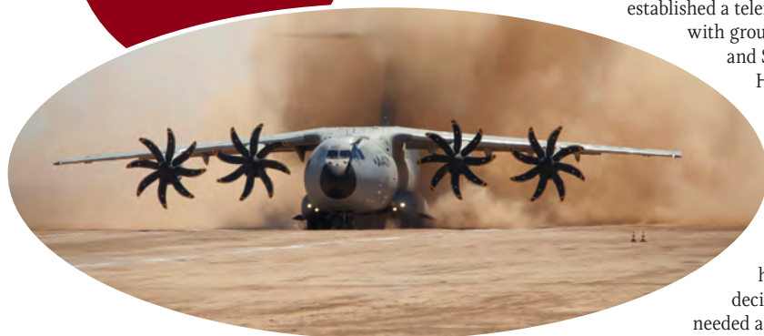
4 // Unpaved runway trials at Ablitas in northern Spain, where MSN2 successfully conducted 25 landings during six flights
