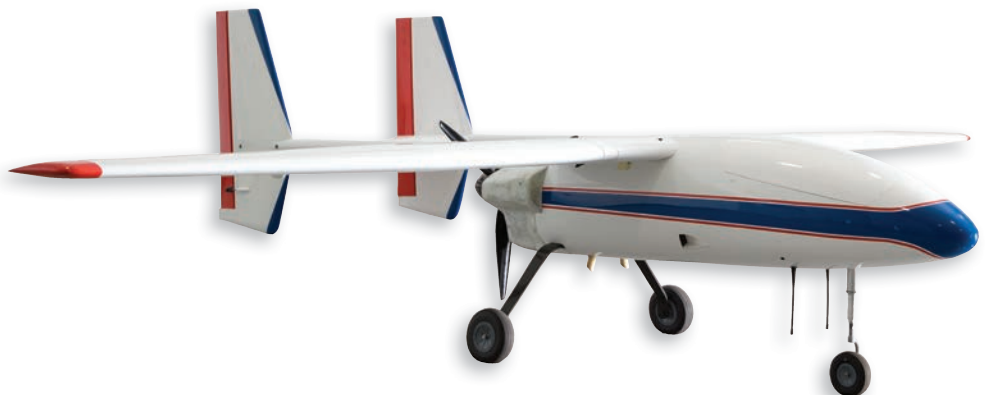
ABOVE: Prometheus, the youngest member of the DLR's research fleet at the Institute of Flight Systems, is a pusher propeller aircraft with a twin-tail unit
