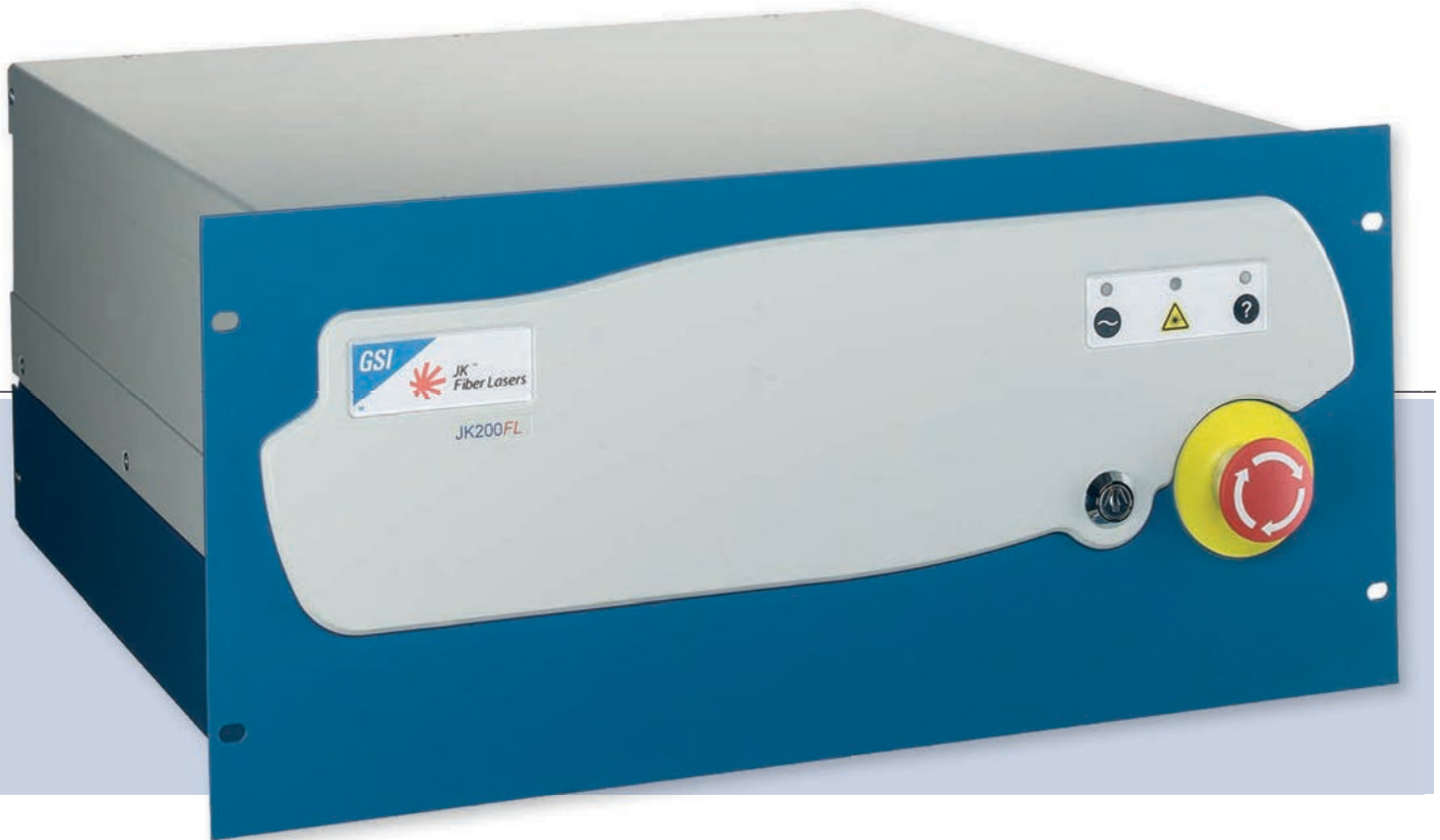
ABOVE: A 200W fiber laser and scanning head were used for trepanning and milling
