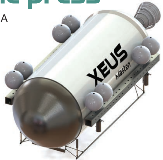
Masten Space Systems' proposed multi-engine dual thrust axis lander
