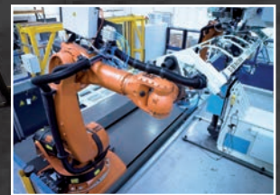
Adaptive Robot Control using Optical CMM or iGPS
