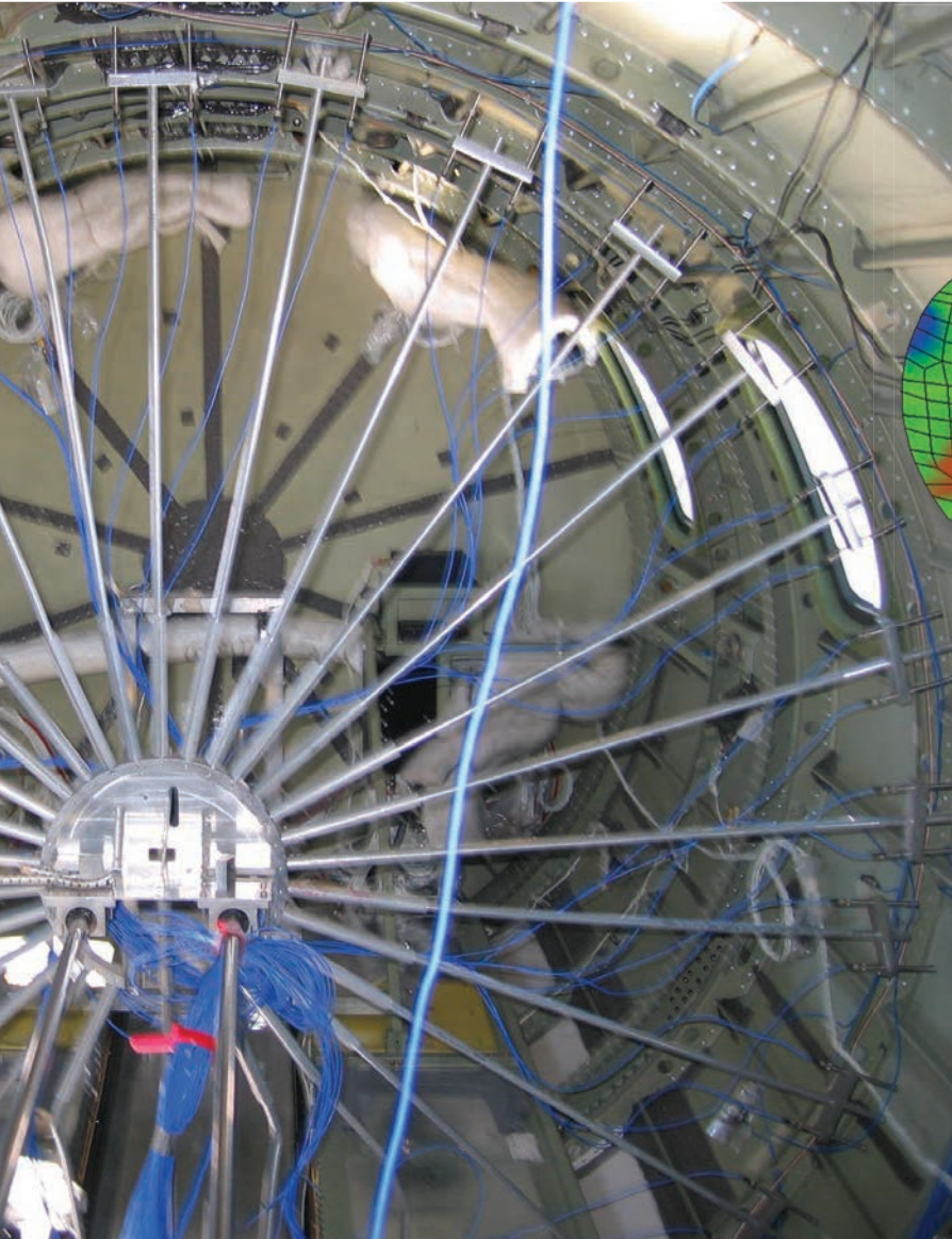
Circular microphone array, PCB Microphone model T130D21
