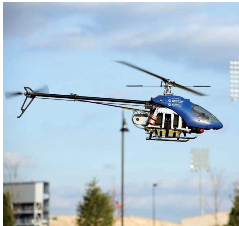
Above: A schematic of the rotorcraft showing the layout of the fuel cell system components. Left: cell-powered rotorcraft in flight. The red battery seen in the picture enables communication with the remote controller
