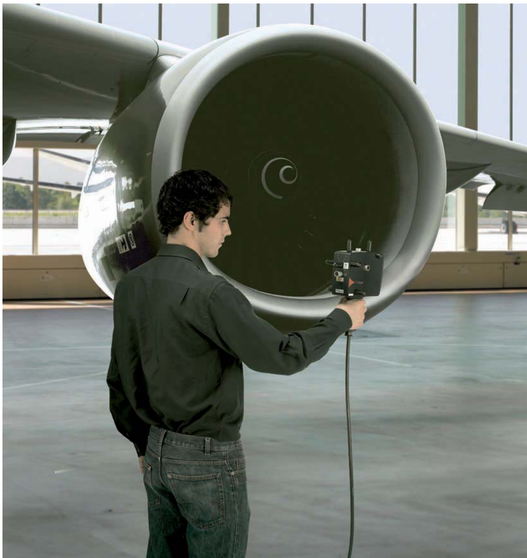
A metrologist using T-scan – The aircraft engine housing is being surface scanned by a handheld Leica T-Scan, which is being tracked Laser Tracker + T-Cam. The tracker is locating one of the retro-reflectors (in silver cylindrical housings) in 3D and the T-Cam (zoom camera) is detecting the angular orientation of the scanner from an image of the LED targets
