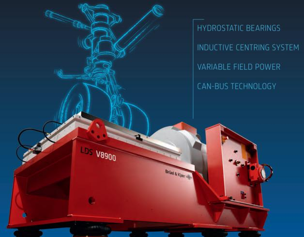
Shake things up with the LDS V8900, the new air-cooled 80 kN shaker from Brüel & Kjær. In a class of its own, this is the air-cooled shaker that meets all your testing needs, now and in the future.
