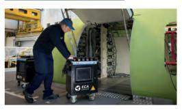
**E**CA Group has developed its novel 'T-Cell' technology to solve challenges with mixed hardware in test benches, component obsolescence and software issues due to operating system upgrades.
