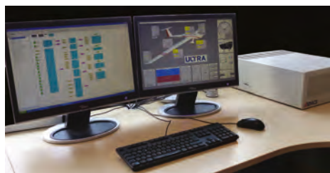
FIGURE 2: Development, simulation and test infrastructure in the ULTRA laboratory with dSPACE real-time systems
