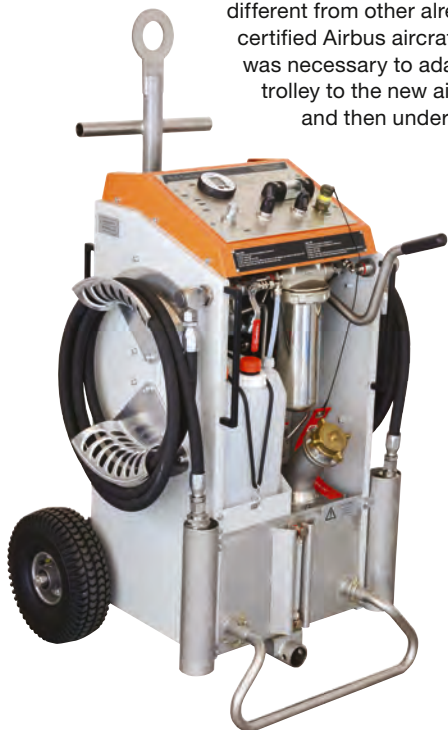
Hand pump for use with the fill-and-drain trolley (right) for the A350XWB's supplemental cooling system
