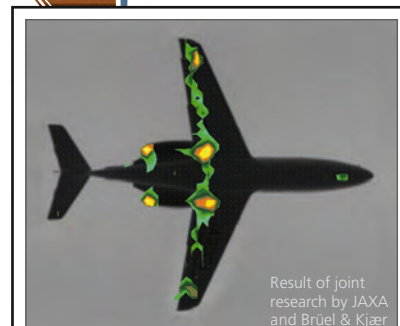
Fast and precise noise source identification
