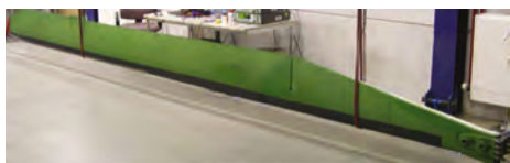
ABOVE: Blade suspended by elastic cords in free-free condition
