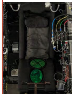
ABOVE: Detail of the Solar Impulse 2's multipurpose seat, including toilet facility (Photo: Solar Impulse/Pizzolante)
