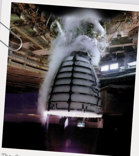
The Space Shuttle main engine is being repurposed as the RS-25 core engine of the new Space Launch System
