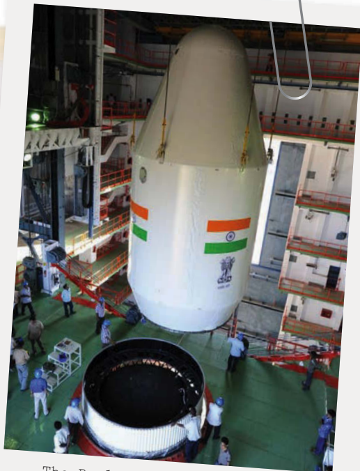
The Payload Fairing is positioned on top of the stacked vehicle and its integrated payload
