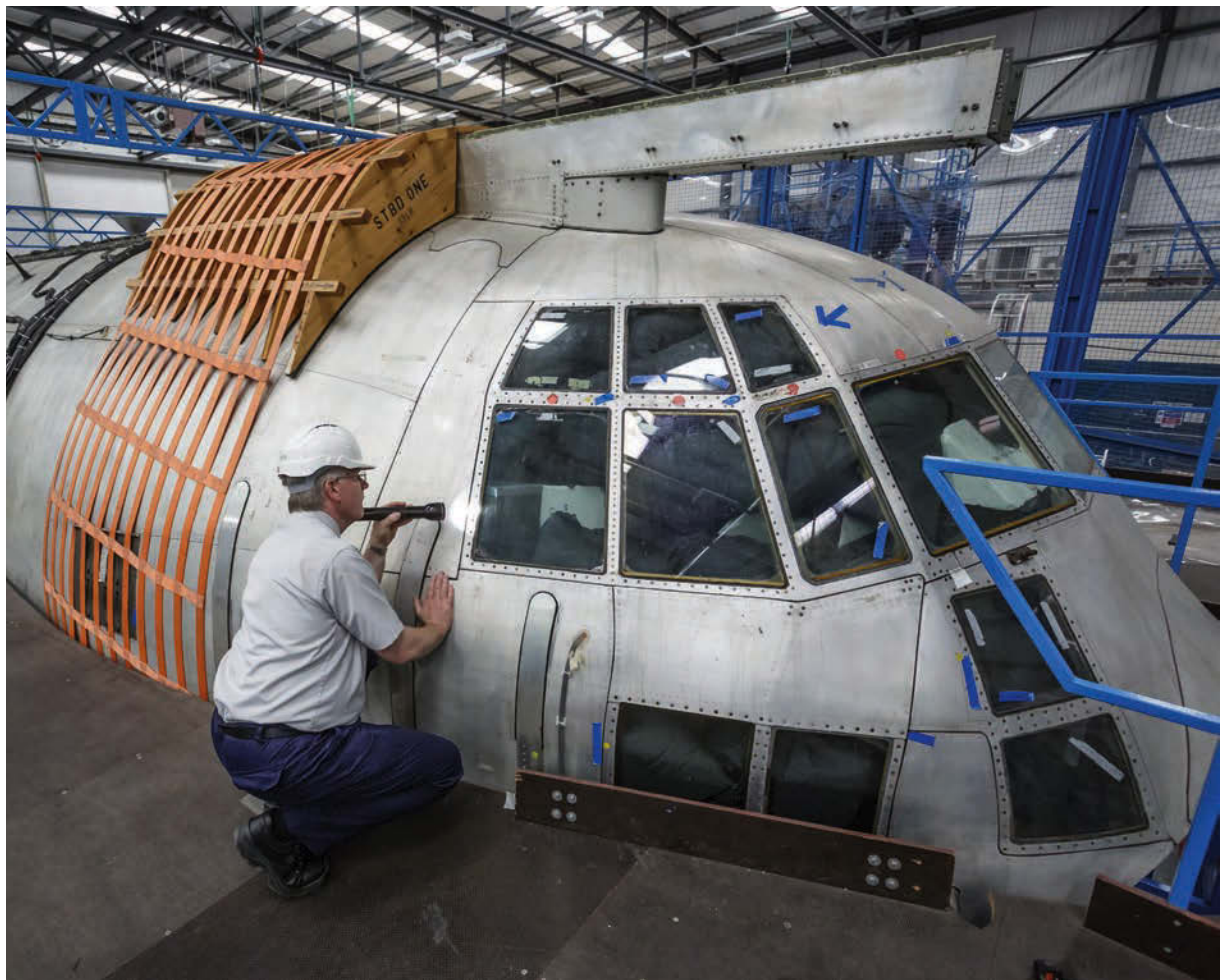
RIGHT: The C-130 fuselage fatigue test rig in Marshall's test hangar
