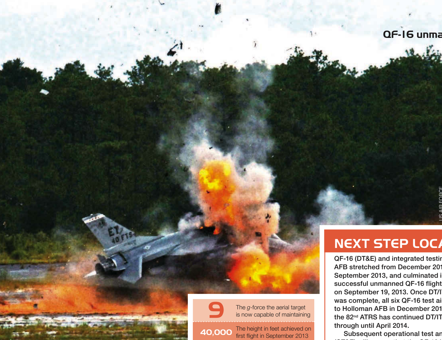
LEFT: An F-16 explodes during tests of the QF-16 Flight Termination System in 2010. The test demonstrated that the FTS design could terminate the flight of a QF-16 immediately with a controlled debris footprint
