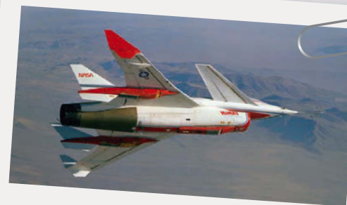
The HiMAT subscale research aircraft, seen here during a research flight in December 1980, demonstrated advanced fighter technologies that have been used in the development of many modern high-performance military aircraft
