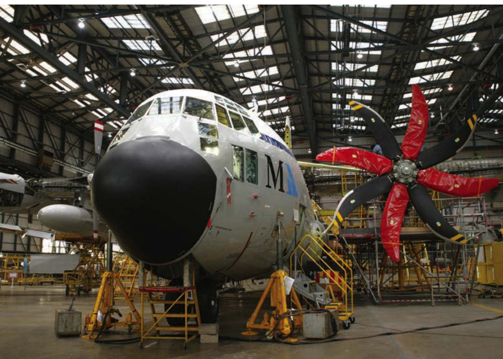
LEFT: The TP400 Flying Test Bed mounted the subject engine inboard on its port wing
