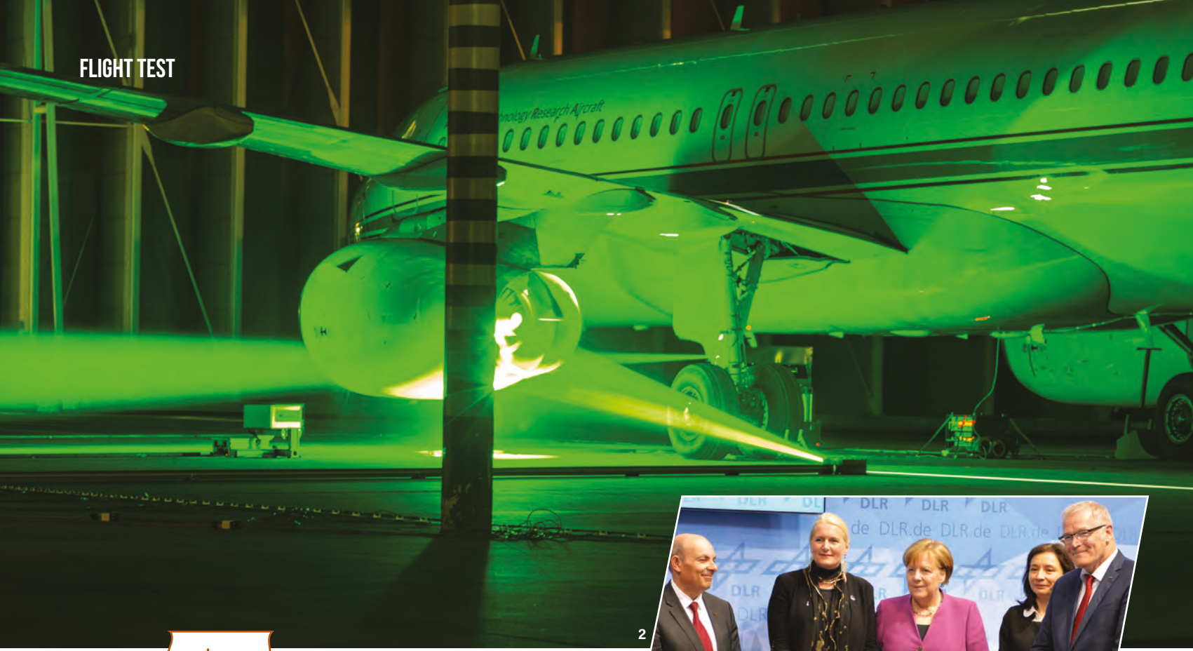
2 // The ATRA A320 during simultaneous engine noise and flow trials
