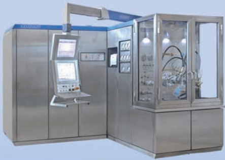
Pump and motor testing (Skydrol)
