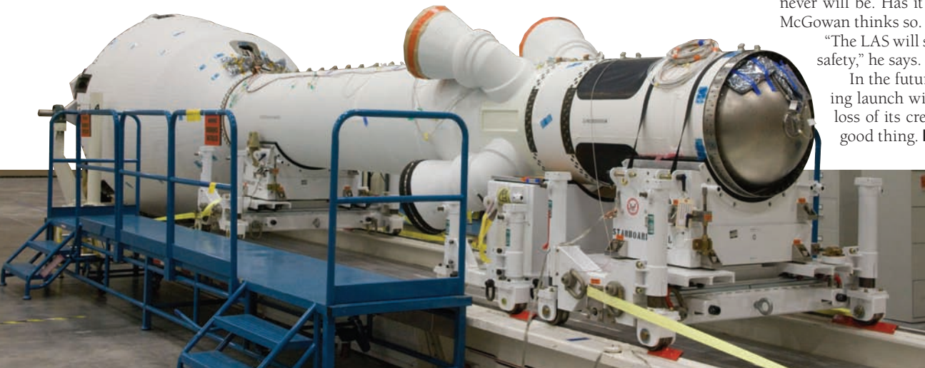
The Launch Abort System's abort motor is connected to the adapter cone assembly at the White Sands Missile Range in New Mexico. Photo credit: US Army White Sands Missile Range
