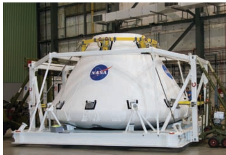
The mock-up Orion crew module that will be used for the Launch Abort System Pad Abort 1 test prior to transport to the White Sands Missile Range in New Mexico (Pictures courtesy: NASA)
