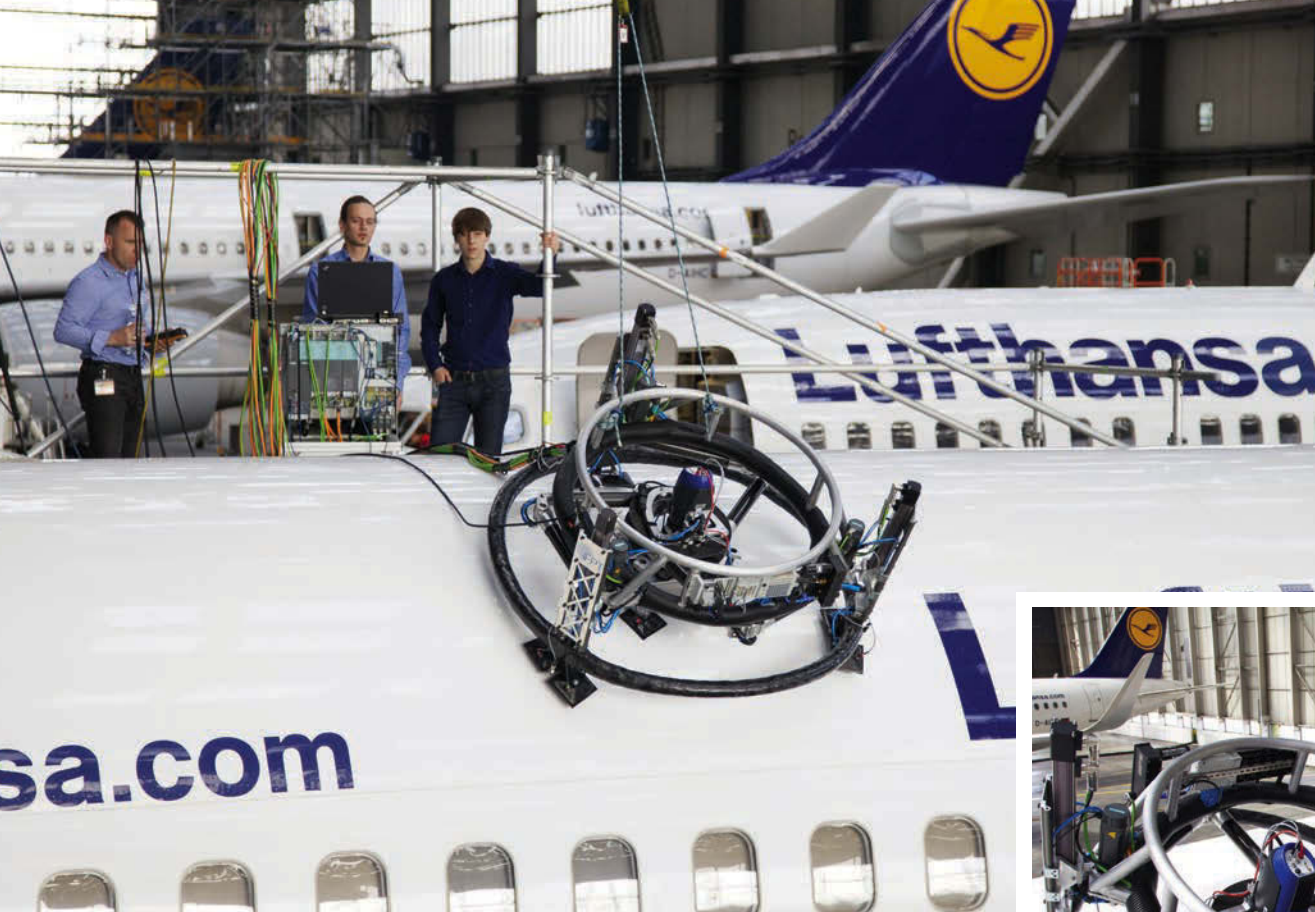
LEFT: The Morfi robot uses active thermography to examine the chemically milled pockets in 737 Classic fuselage skin plates
