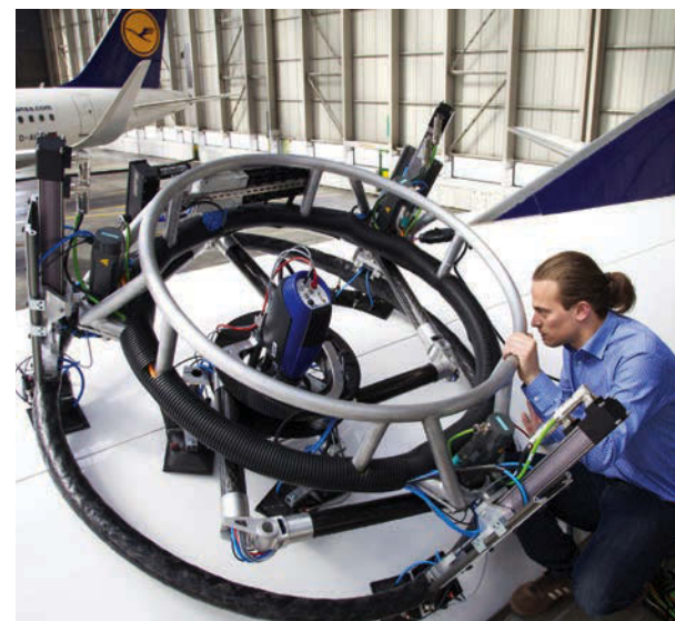
ABOVE: Lufthansa Technik has developed a prototype robot to inspect Boeing 737 Classic fuselage panels
