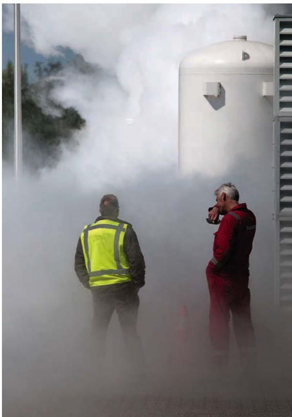
RIGHT: Two experts flush a 33,000 liter liquid nitrogen tank
