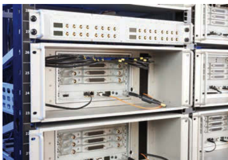
FAR RIGHT: PAK MKII acquisition units in the used 19in racks
