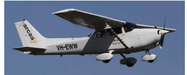
ABOVE: The Cessna 172 used in the Safe Skies program to demonstrate UAS use in shared airspace
