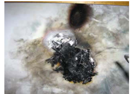
CFC-Part after Direct Lightning application with 100kA
