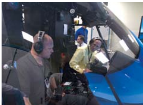
US Marine Corps pilots test the cockpit controls in a mock up of the new VH-71 presidential helicopter
