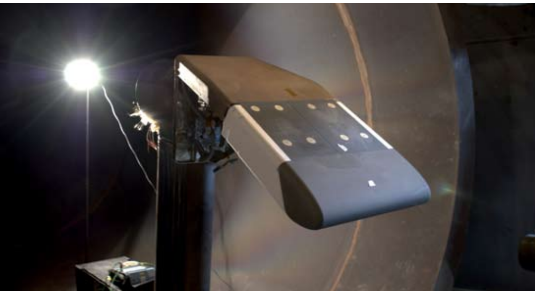
First configuration of the wing model fitted with an actively refrigerated metal leading edge and carbon-carbon panels
